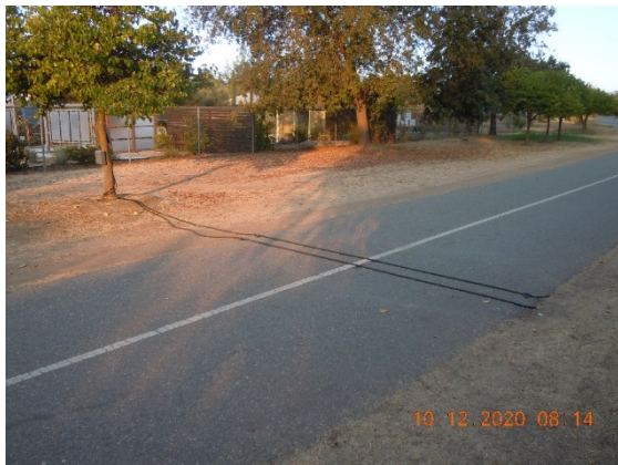
Portable Bike and Pedestrian Trail Counter along the Dry Creek Trail
